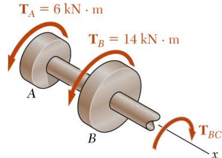
$$\sum M_x = 0 = (6 \text{ kN} \cdot \text{m}) + (14 \text{ kN} \cdot \text{m}) - T_{BC}$$
