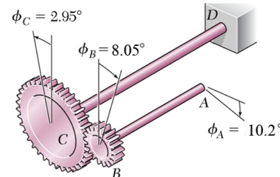
$$\phi_{A/B} = \frac{T_{AB}L}{J_{AB}G} = \frac{(61.8 \text{ Nm})(0.6 \text{ m})}{\frac{\pi}{2}(0.0095 \text{ m})^4 (77 \times 10^9 \text{ Pa})} = 0.0376 \text{ rad} = 2.15^\circ$$
