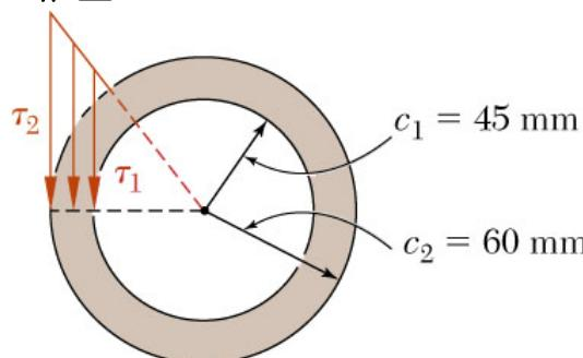
$$J = \frac{\pi}{2} (c_2^4 - c_1^4) = \frac{\pi}{2} [(0.060)^4 - (0.045)^4] \\ = 13.92 \times 10^{-6} \text{ m}^4$$
