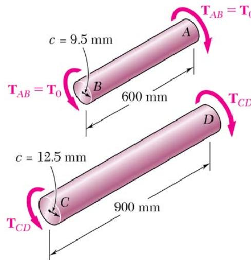
$$\tau_{\max} = \frac{T_{AB}c}{J_{AB}} \quad 55 \times 10^6 \text{ Pa} = \frac{T_0(9.5 \times 10^{-3} \text{ m})}{\frac{\pi}{2}(9.5 \times 10^{-3} \text{ m})^4}$$
