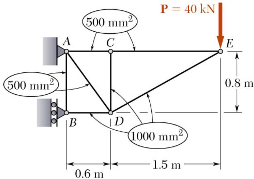
Members of the truss shown consist of sections of aluminum pipe with the cross-sectional areas indicated. Using  $E = 73$  GPa, determine the vertical deflection of the point  $E$  caused by the load  $P$ .
